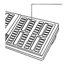
Memory buttons are the buttons with labels other than line or Handsfree buttons. Memory buttons store telephone numbers or feature codes to give you one-touch dialling or feature activation. You can change the function of a memory button by programming it with a new number or feature.
